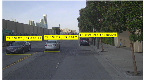
Fig. 3: Image of the PandaSet dataset with bounding boxes for cars based on the YoloV4 algorithm. For simplicity, 3 out of a total of 26 recognized cars are shown. The CS of YoloV4 and \kappa (DS) are given for each of these objects. The detection score here correlates with the CS depending on the resolution of the respective object.
