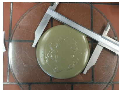
(b) Measuring the slump flow diameter
