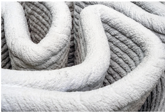
(a) Layers of printed concrete
