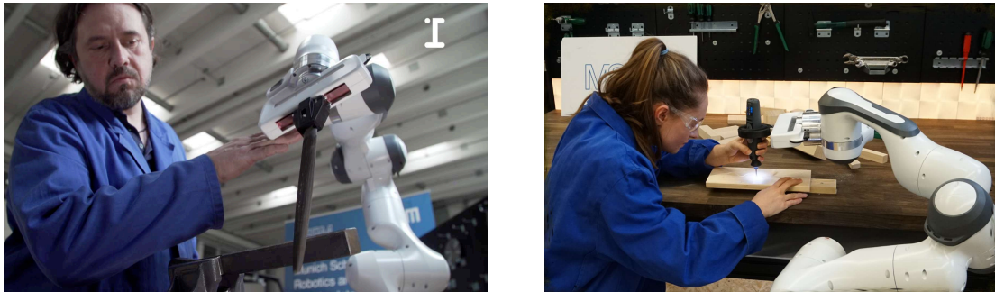
Figure 1.6: Human-robot interaction. Left: Safety-enhancing speed modulation in the Future of Work demonstrator; Right: Precision-improved co-manipulation in wood engraving.
