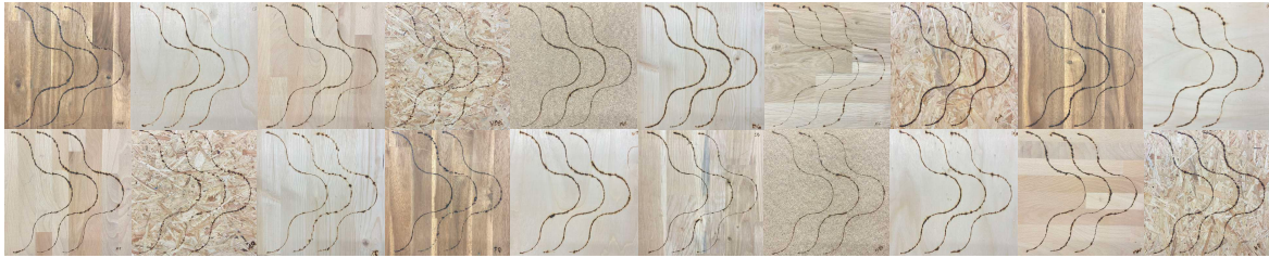
Figure 4.36: Pyrography user study results; twenty participants utilized three distinct modes to produce uniform lines on twenty wooden plates. The lines on the left, center, and right of each plate correspond to mode 1, mode 2, and mode 3, respectively.
