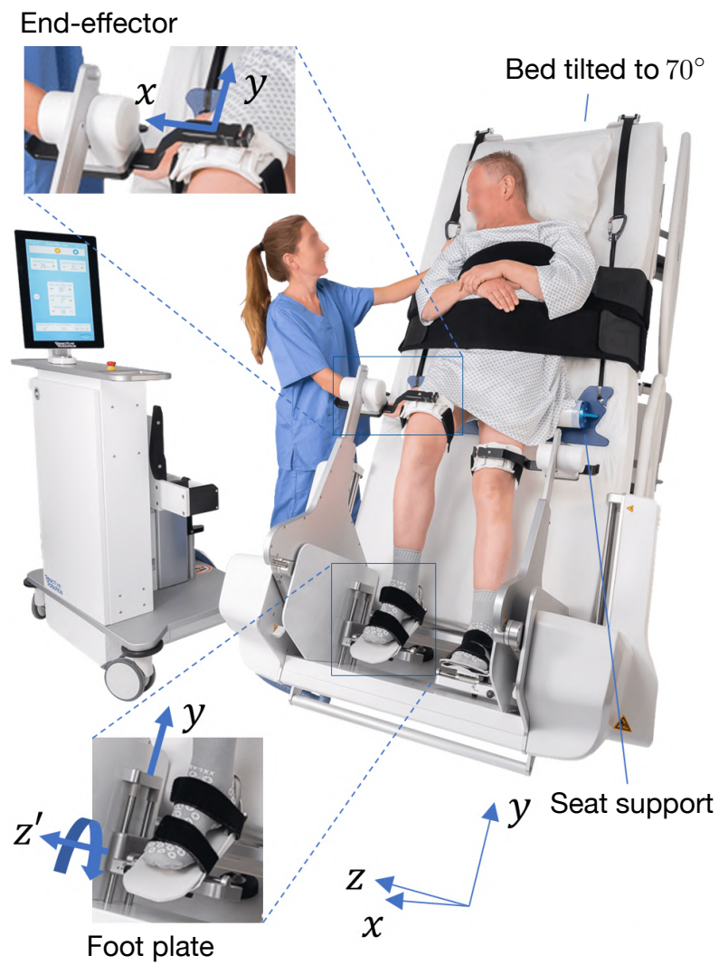
Figure 4.53: Various components of the lower-limb movement rehabilitation robot VEMOTION, featuring the proposed innovative Assist-As-Needed policy.
