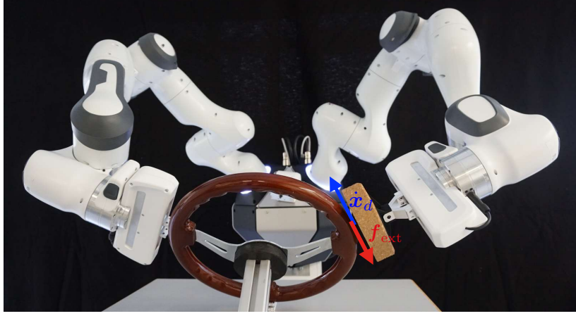
Figure 5.11: A tank provides the required power -\dot{x}_d^T \mathbf{f}_{\text{ext}} to control motion on a frictional surface.
