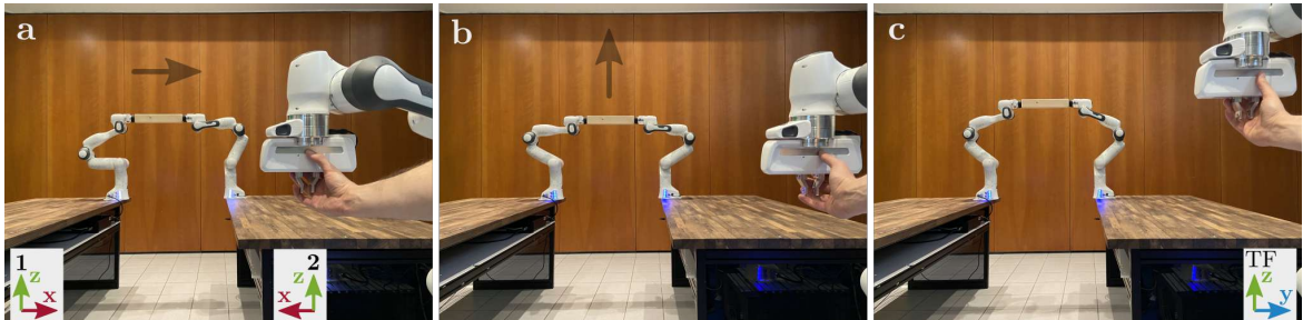
Figure 3.22: Experiment 2 – An operator is remotely manipulating the object by moving the guiding robot in the yz -plane.
