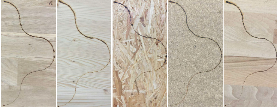
Figure 4.35: Automated pyrography with an impedance-controlled robot along a predefined path at a constant speed. The wood burner temperature intentionally drops by a quarter in the middle, resulting in a fainter marked line thereafter.
