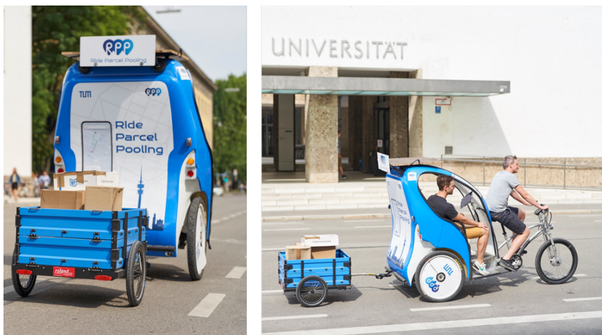
Figure 6.6: RPP rickshaw (prototype for the integrated transportation of passengers and freight).
