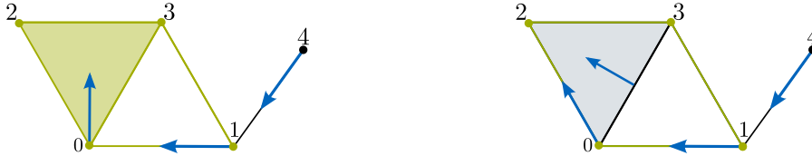
Figure 8: Left: Generalized discrete gradient (blue) with corresponding descending complex (green). Right: lexicographic gradient refinement (blue) with corresponding descending complex (green).
