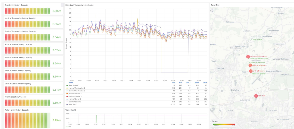
Figure 4.3: Example of how the dashboard for the GeoSensor Network at the Kalterbach is displayed on Grafana
