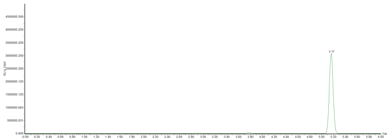
Figure 53: Fluorescence (290/410 nm) in the first 6 min of the HRMS run of (1a) before biological degradation (green line).
