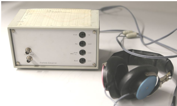
Figure 1. Custom free-field equalizer for Beyerdynamic DT48 headphones [1].
