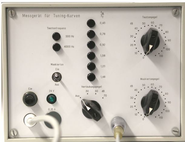
Figure 2. Custom device for measuring psychoacoustic tuning curves.
