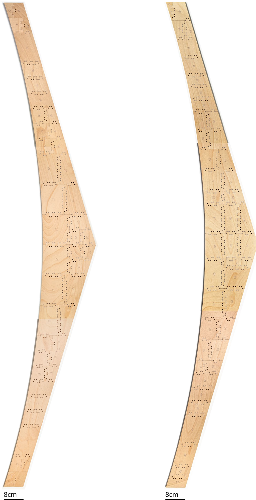
Figure 42: The pitched cambered beam, the first segmentation layer on the left, and the second on the right.
