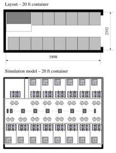
Figure 2. Comparison of the layout drawing with the simulation model of the 20 ft container.
