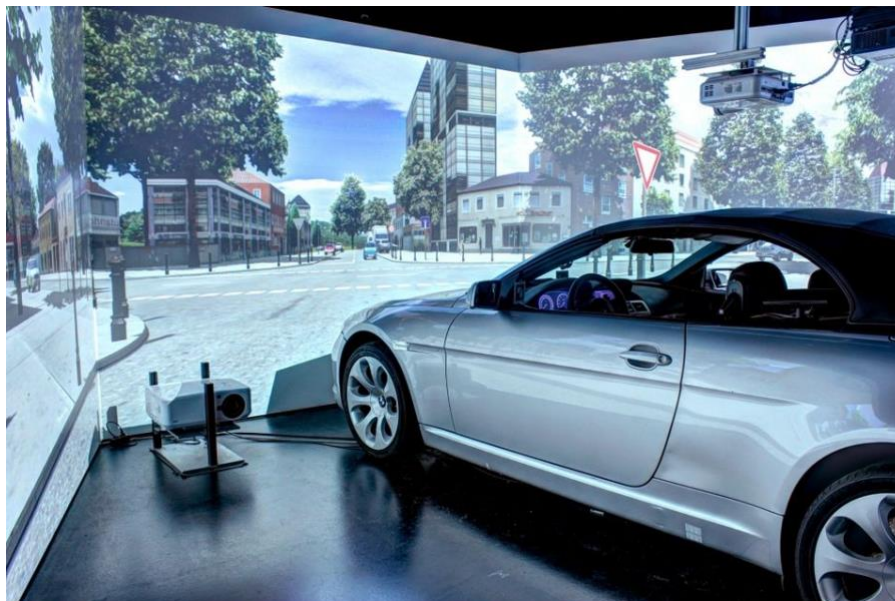
Figure 5.5: Fix-base driving simulator of the Chair of Ergonomics at Technical University of Munich used in this study.
