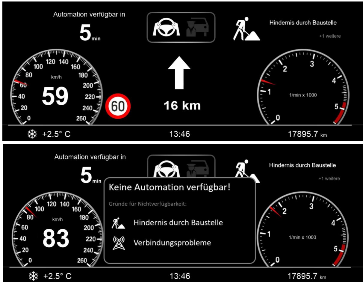
Figure 5.6: The picture above shows the HMI display for AC2 with the ADS being non-available. The duration until the ADS became available is in the top left corner with the following text: “Automation available in 5min”.
