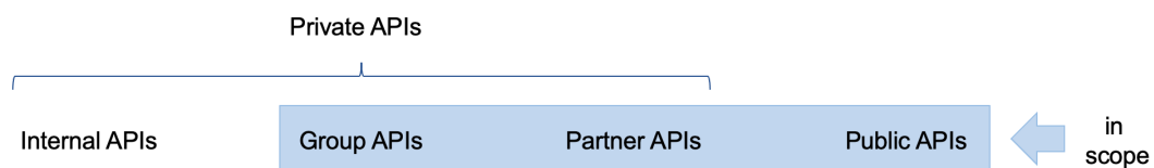
Figure 2.3.: Overview of different Web API accessibility categories (De, 2017; Jacobson et al., 2012; Doerrfeld et al., 2015), highlighting the scope of this dissertation.
