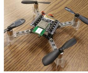
Figure 10: CrazyFlie 2.0 quadrotor helicopter with UWB expansion.
