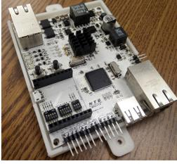
Figure 8: Custom anchor with ARM Cortex M4 processor and UWB slot.
