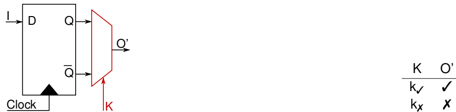
(b) Using a multiplexer behind FFs with key selector bit K [KCK20]
