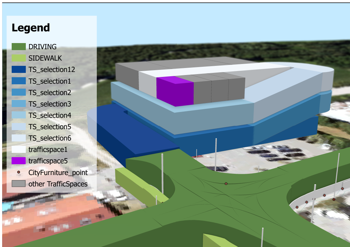
Figure 4.27.: Parking Garage - Routing from Parking Spot: The routing starts at the parking spot in purple and follows the blue colour gradient to the exit TrafficSpace in dark blue.
