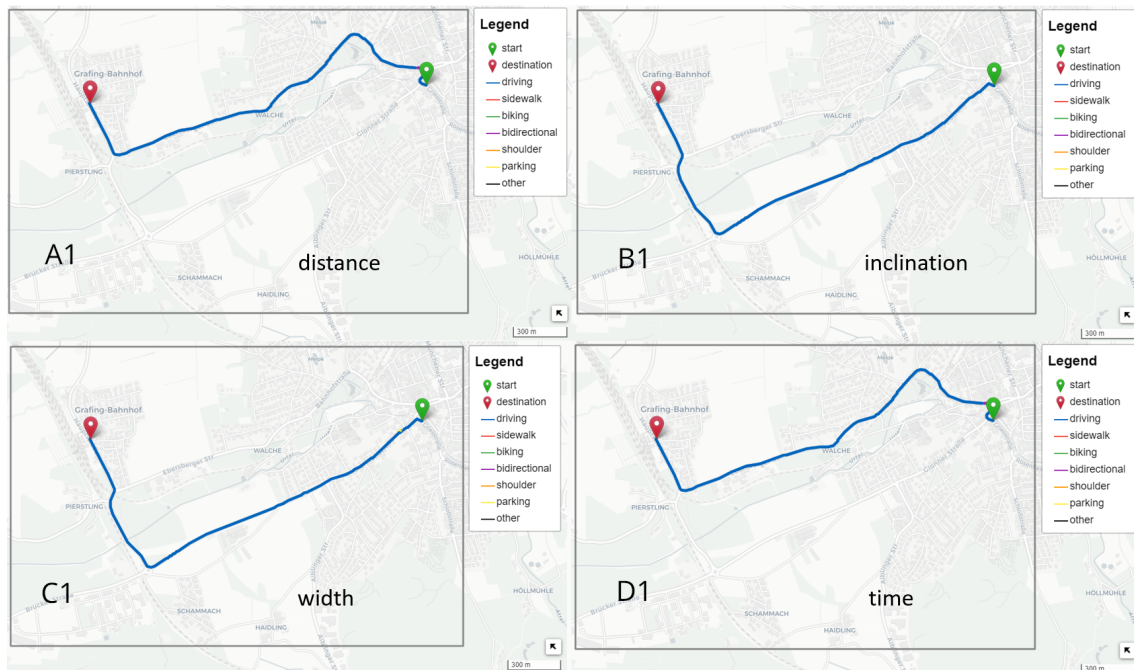
Figure 4.12.: Dijkstra Shortest Path Combination 1 Map Display
