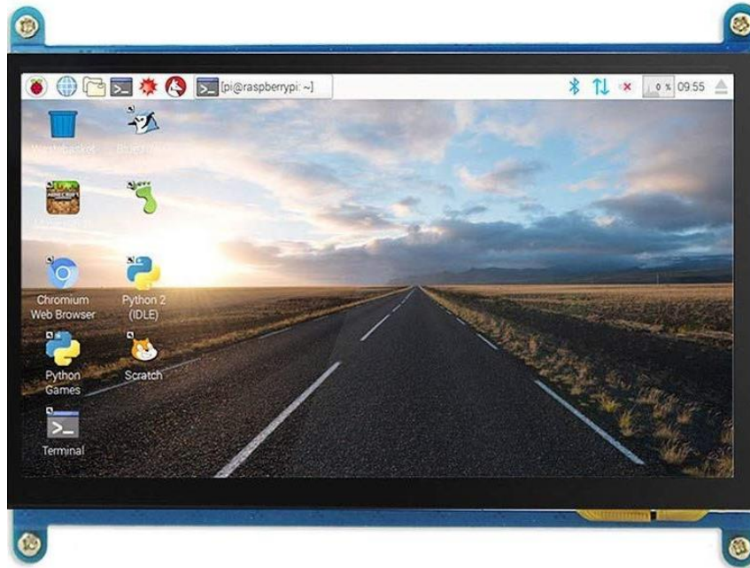
Figure 9: 7-inch IPS capacitive touchscreen.
