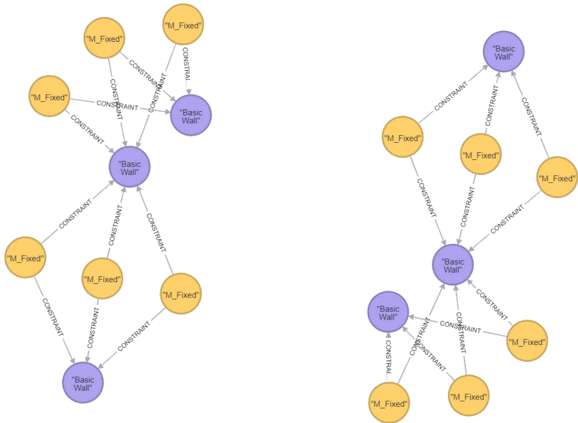
Figure 33: The graph representation of design constraints which is created for horizontal distances between window and walls in the rooms called "Office".
