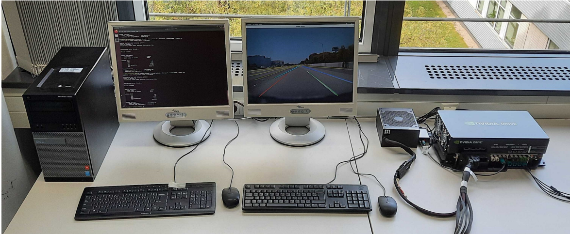
Figure 7.6: The mapping experimental setup using the Nvidia Drive AGX. On the left is the host computer, and on the right is the Nvidia Drive AGX Xavier with the power adapter. Both are connected to a monitor and other peripherals.
