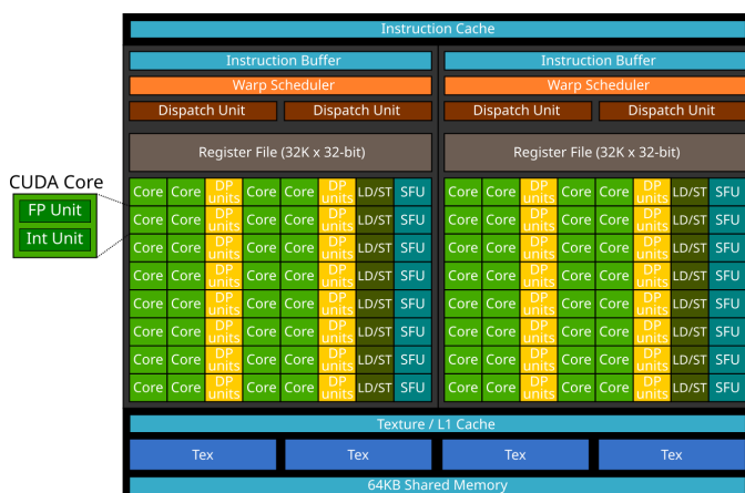
Figure 5.1.: Nvidia GP100 Streaming Multiprocessor. The image was drawn according to the description given in [91].
