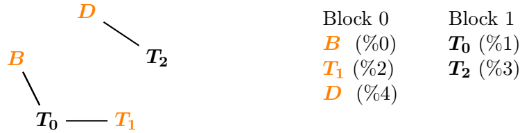
Figure 6.5.: Graph coloring and the operands’ assignment to shared memory blocks for Eq. 6.3.
