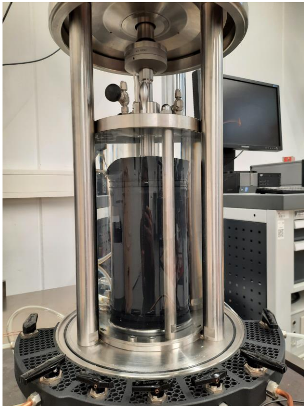
Figure 6.4: Photo documentation of sample preparation of triaxial samples
