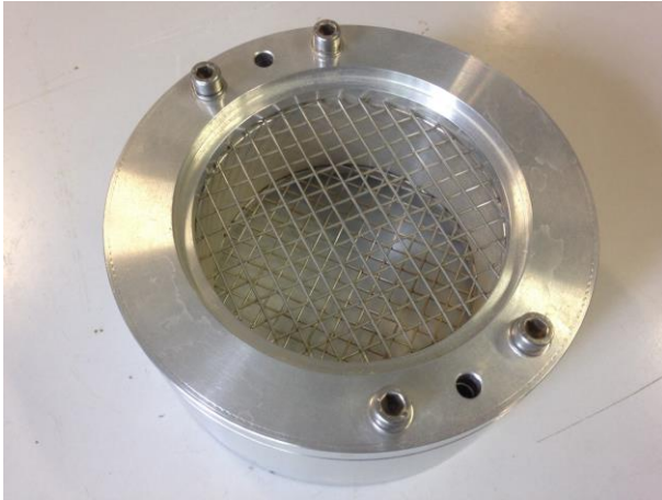
(a) (b) Figure 6.3: (a) Photo of the diffuser and (b) photo of the perforated plate and shutter
