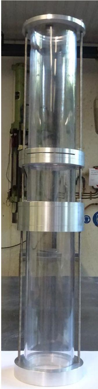
(a) (b) Figure 6.2: (a) Schematic sketch and (b) photograph of the sand pluviator
