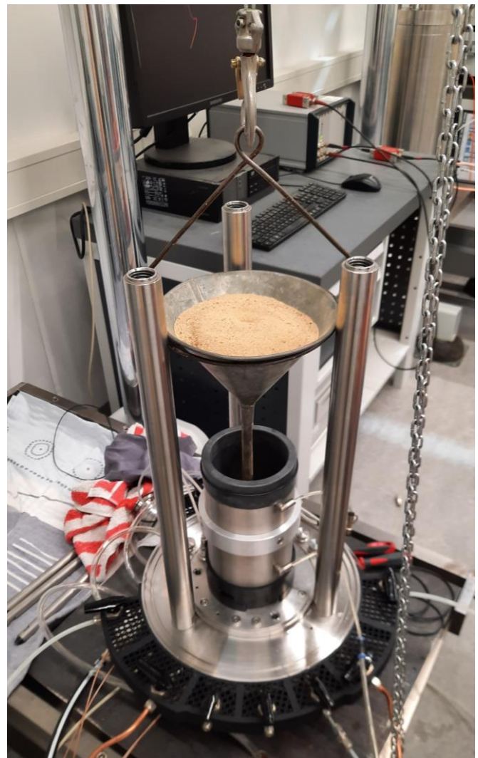
Figure 4.7: Sample preparation by (a) air pluviation and (b) dry funnel deposition method in the triaxial test setup
