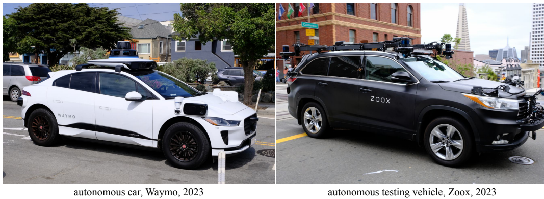
Figure 2.4. Vehicles by Waymo and Zoox equipped with autonomous driving sensors and features. The pictures were captured in the streets of San Francisco, California, in June 2023. The Waymo car on the left has no driver and can offer autonomous rides to selected users, operating as a robot taxi. Vehicles like the retrofitted white Jaguar I-Pace shown are equipped with many sensors in various housings, especially around the roof area. Zoox is developing a mini-bus without driving controls on board and is testing on public roads with retrofitted Toyota Highlander SUVs equipped with multiple sensor rigs featuring numerous sensors, especially around the roof and front of the vehicle. While the sensor configuration between the two is different, both companies opted for multiple LiDARs, cameras, and radars. The images have been anonymized, hiding license plates and vehicle identifiers.
