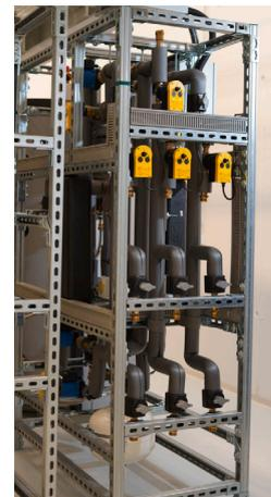
Fig. 4. Bidirectional heat and cold transfer station: a) schematic drawing; b) setup at the CoSES laboratory.
