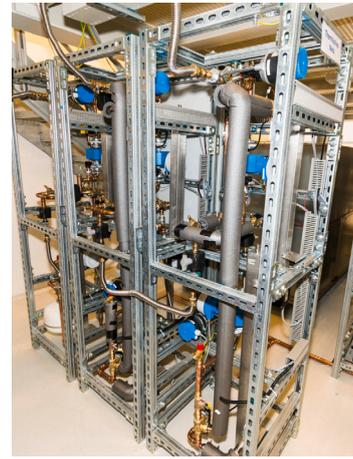
Fig. 3. District heating and cooling grid emulator: a) schematic drawing; b) setup at the CoSES laboratory.
