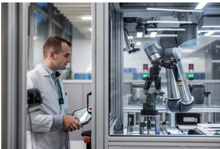
Figure 1.2: Traditional lead-through programming with the human holding and interacting with the teach pendant to program robot sequences or positions.
