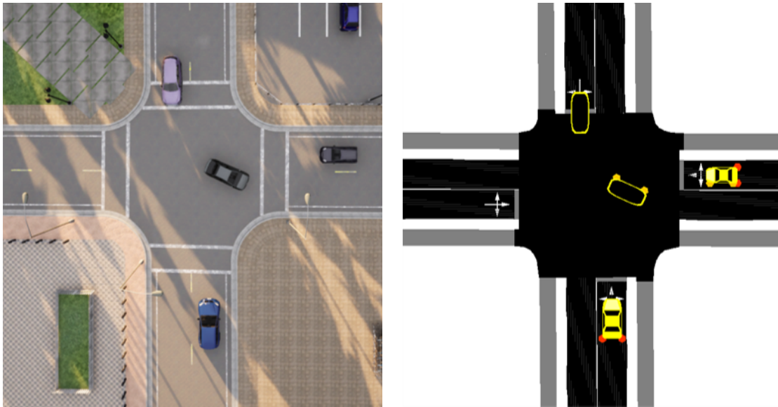
Figure 6.3: A scenario in the CARLA simulator (left) and SUMO simulator (right). The states of the ego vehicle (blue car) and other road users are synchronized between CARLA and SUMO (graphic from [Zha+22a], ©2022 IEEE).
