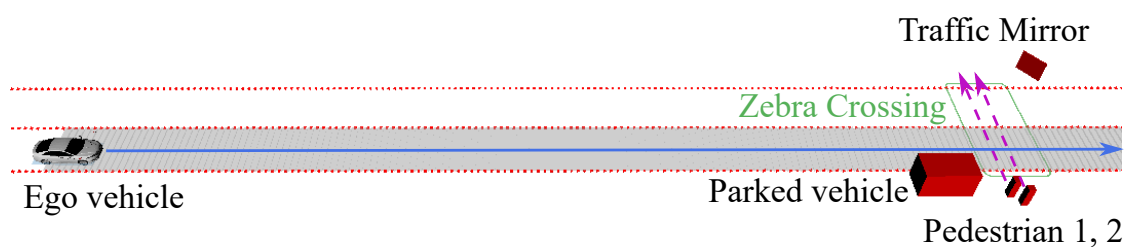
Figure 3.14: Scenario C: Ego vehicle driving through a crosswalk with occlusion caused by a parked vehicle. Scenario D: Two pedestrians intend to cross the road, but their views are blocked (graphic from [Zha+22c], ©2022 IEEE).
