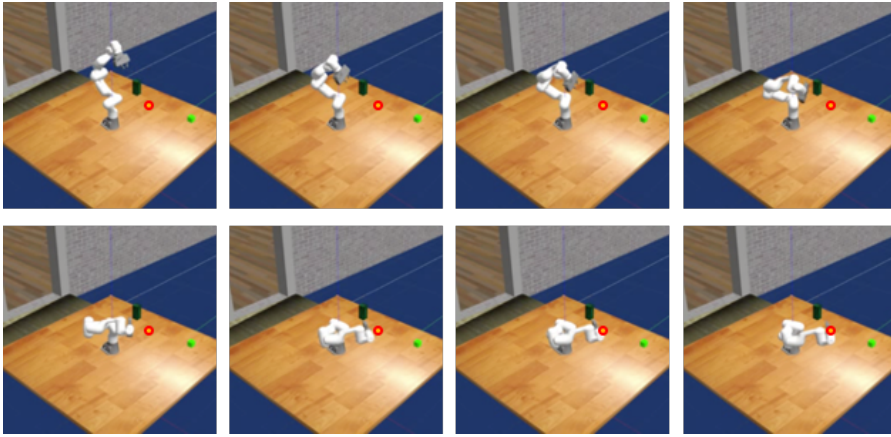
Figure B.4: Single obstacle avoidance: cube. The red circle is the goal.
