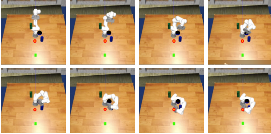
Figure B.3: Multiple Obstacle Avoidance: Unsuccessful Trial. The red circle is the goal. The robot collides with the cylinder at the end of the execution.
