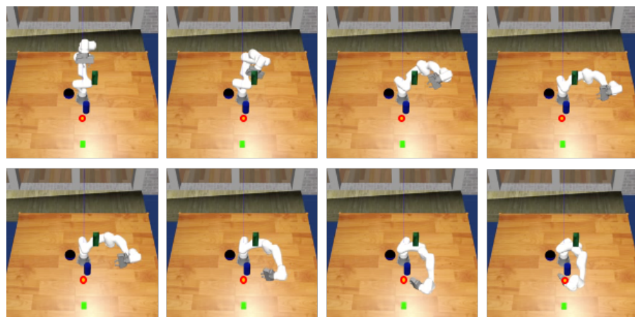
Figure B.2: Multiple Obstacle Avoidance: Successful trial. The red circle is the goal.
