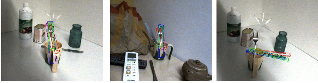
Fig. 5.10 S^2P^3 Qualitative Results with Occlusions: Zoomed-in from Fig. 5.9. Before and after self-supervision. The projected bounding boxes in blue, red, and green represent the ground-truth 6D object poses, the results before and after applying self-supervision, respectively.
