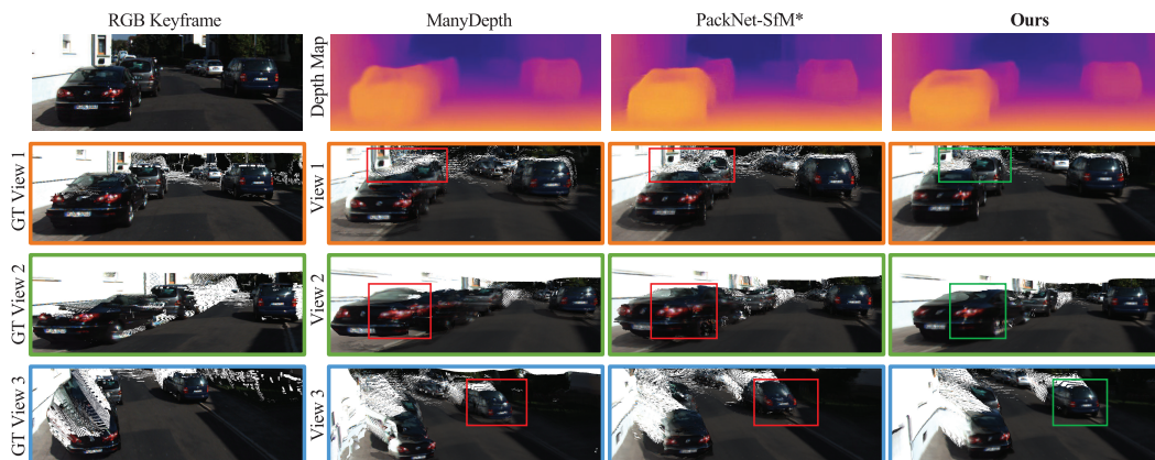
Fig. 2.7 Qualitative Depth Consistency: Qualitative reconstructions using five sequential depth predictions reveal distinct differences. Both ManyDepth [171] and PackNet-SfM* [53] with velocity semi-supervision, exhibit artifacts like "flying pixels" in View 1, ghosting effects in View 2, and distorted objects in View 3. These issues stem from temporal inconsistencies. While these may not be evident in single-frame depth predictions, they become prominent when the viewpoint shifts. Our approach substantially reduces these visual discrepancies.
