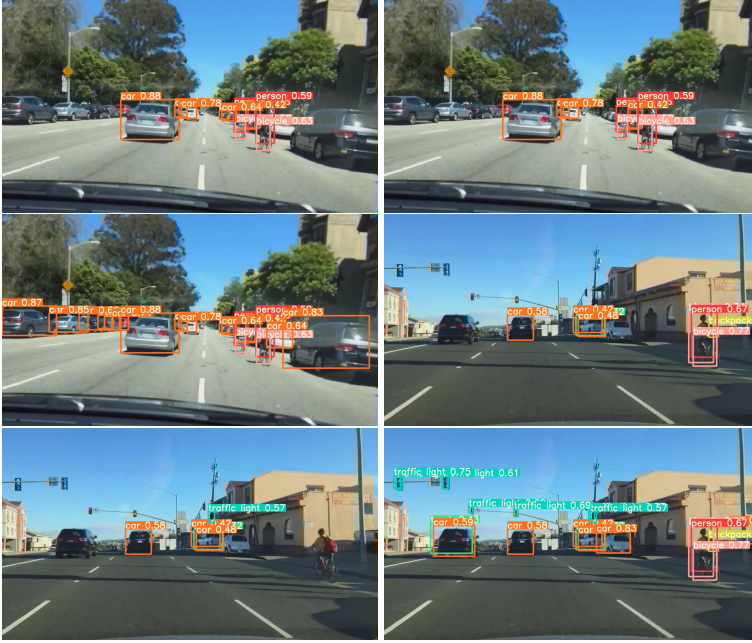
Fig. 6. Comparison of our prediction, ground-truth in attention-based object detection and not using attention-based object detection on BDD-A test set. (Failed cases.) Left: Our prediction; Middle: Ground-truth; Right: Object detection without driver attention. Better view in colors.
