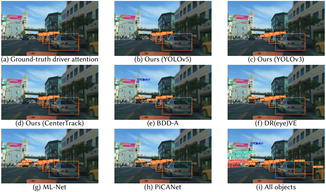
Fig. 5. Comparison of attention-based object detection using different models. (a) Ground-truth attention; (b-d) Predictions using our framework with different backbones; (e-h) Predictions using models [8, 26, 34, 54]; (i) Object detection without driver attention.
