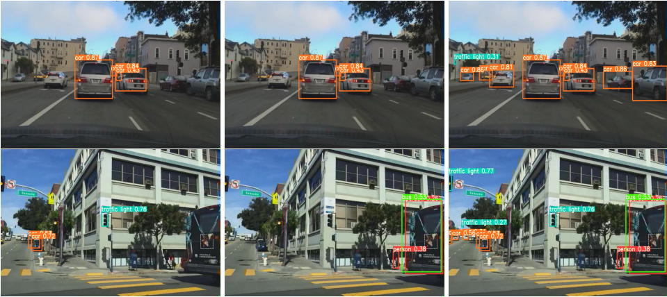
Fig. 11. Comparison of our prediction, ground-truth in attention-based object detection ( Th = 0.5 ) and not using attention-based object detection on BDD-A test set. (Second line is failed case.) Left: Our prediction; Middle: Ground-truth; Right: Object detection without driver attention. Better view in colors.
