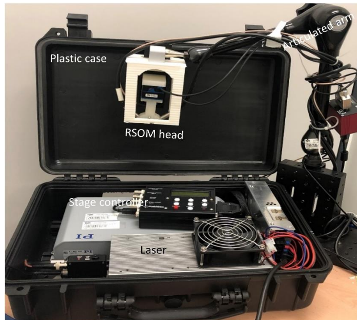
Figure S1. Picture of the portable RSOM imaging system. The laser source and the stage controller are contained within a plastic suitcase, creating a controlled laser safety environment during the measurement of the participants with or without diabetes mellitus.
