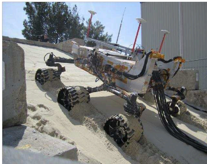
Figure 2.1: Mars Science Laboratory (MSL) engineering model tested on dry, loose sand taken from [4].
