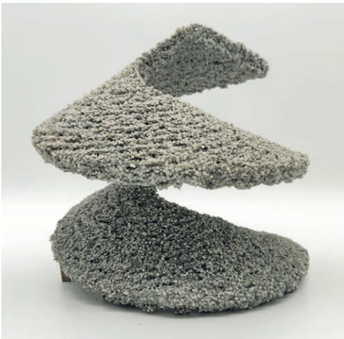
Bild 13: Helix, hergestellt durch Selective Cement Paste Intrusion | Fig. 13: Helix, manufactured by Selective Cement Paste Intrusion
