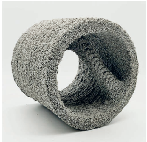
Bild 14: Innen verstreutes Rohr, hergestellt durch Selective Cement Paste Intrusion | Fig. 14: Pipe with internal structures manufactured by Selective Cement Paste Intrusion
