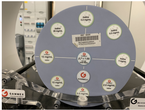
(a) Gammex phantom with iodine inserts (0.2 - 20 mgI/mL).
