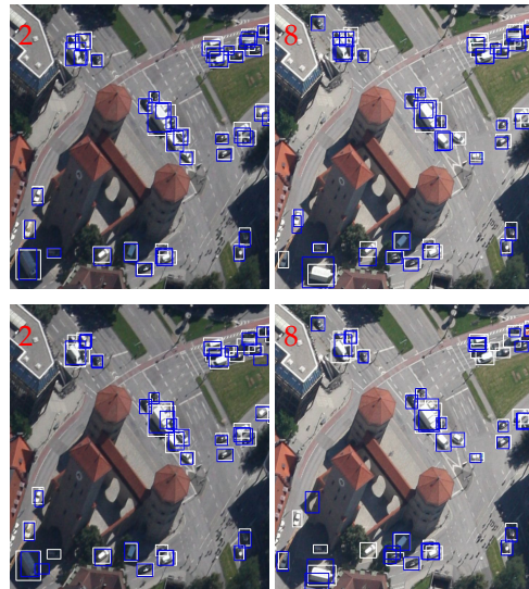
Figure 19. Tracking results by AerialMPTNet (top row) and SMSOT-CNN (bottom row) on the frames 2 and 8 of the “MunichCrossroad02” sequence of the KIT AIS vehicle dataset. The predictions and ground truth bounding boxes are depicted in blue and white, respectively.
