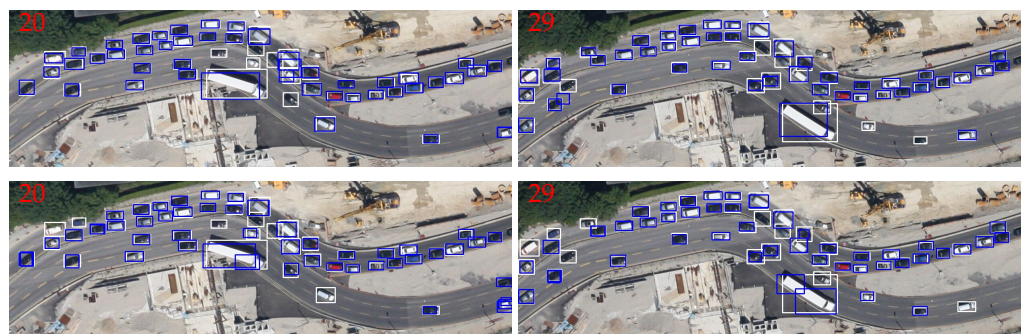
Figure 20. Tracking results by AerialMPTNet (top row) and SMSOT-CNN (bottom row) on the frames 20 and 29 of the “MunichStreet04” sequence of the KIT AIS vehicle dataset. The predictions and ground truth bounding boxes are depicted in blue and white, respectively.
