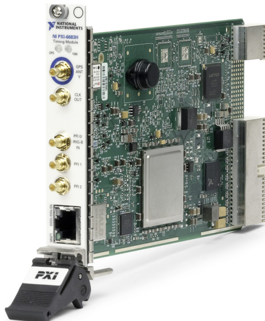
Figure 2.1: The NI PXIe 6683H timing and synchronisation card used in CoSES PXIe controllers. [93]
