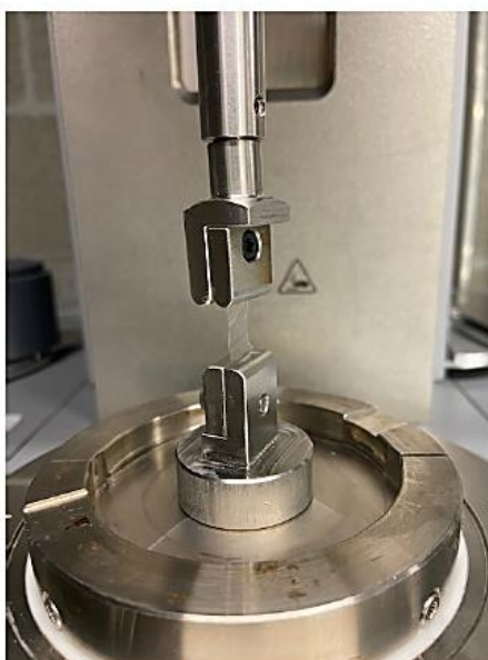
Figure S7. Experimental setup used to determine the tensile strength of the films.
