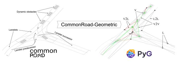
Fig. 1: Our package serves as a bridge from CommonRoad to PyTorch-Geometric. The abbreviated graph labels refer to the heterogeneous node and edge entities of our unified traffic graph structure covered in Section III-A.
