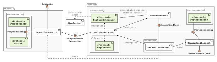
Fig. 6: High-level software architecture for cr-geo shown as a UML 2 component diagram [33].
