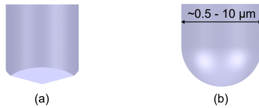
Figure 2.20: Different indenters for nanoindentation, Berkovich tip (a) and the spherical tip (b).
