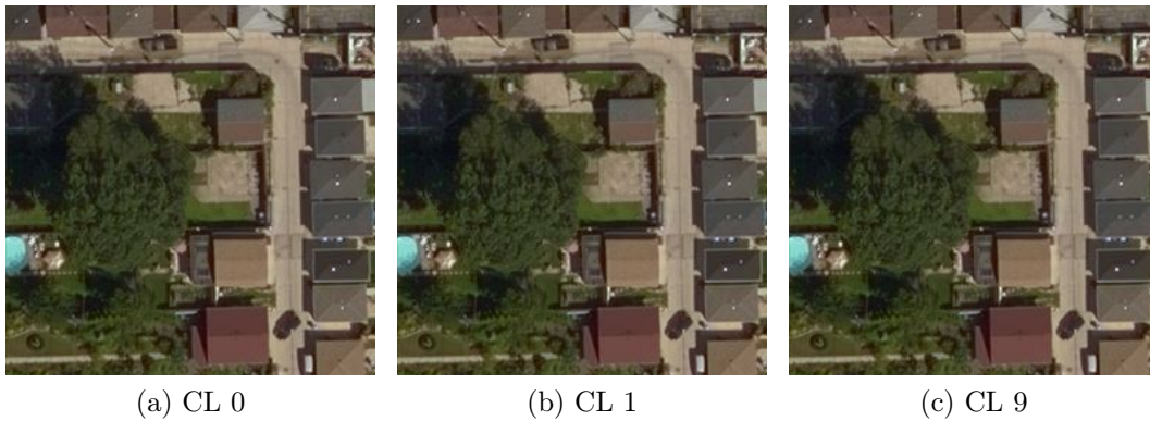
Figure 4.6: The image format PNG is able to hold up to three channels (plus an alpha band) with a maximum bit depth of 24-bit in total. Additionally, ZLIB is used to compress the data to reduce the memory footprint. The compressor has nine levels in total, while the lowers indicates that no compression is applied, and one sets the concentration on the performance. Level nine focuses on maximum compression. Furthermore, PNG is a lossless image format, therefore, the source data can be reproduced by the compressed version without any error. This is also the reason why there is no visible difference between the sub-figures. This figure has been first published in [P11].
