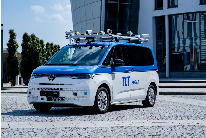
Figure 6.5: Research vehicle EDGAR [308], which is based on a Volkswagen T7 vehicle and has been extended by sensors and computing hardware to fulfill requirements for automated driving in urban environments with a safety driver.
