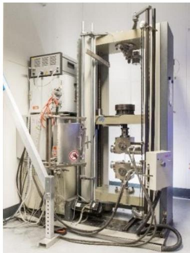
Figure 4-2: Zwick 1484 tensile compression testing machine (Photo: Mr. Hase)
