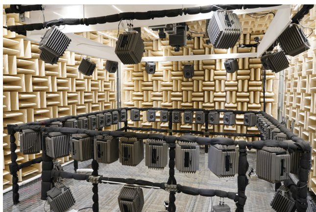
FIG. 1. (Color online) Loudspeaker array in a 10 m × 6 m × 4 m anechoic chamber. The loudspeakers are placed on a 4.8 m × 4.8 m frame in 10° azimuth steps and equalized in level, delay, and phase.
