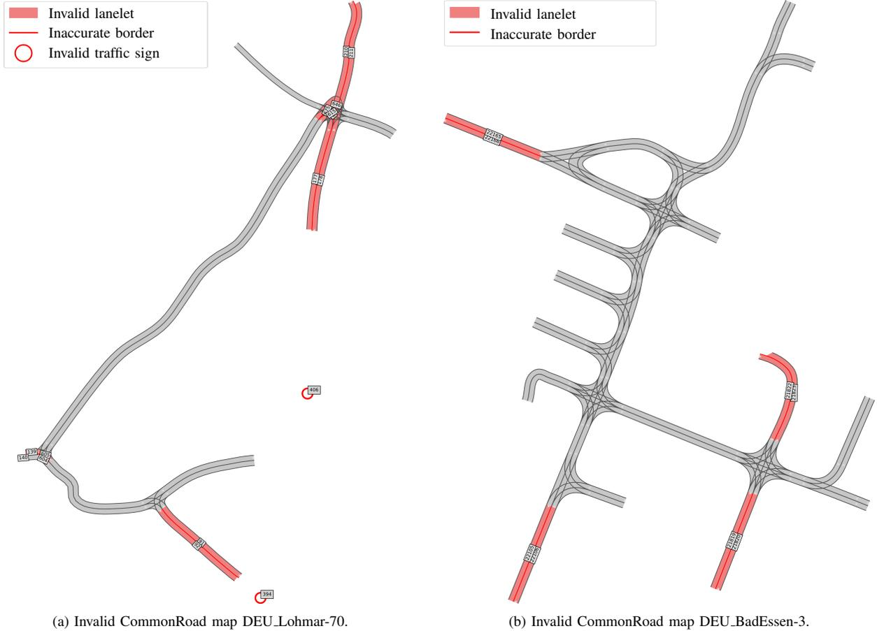
Fig. 6: Map errors of two CommonRoad maps consisting of several intersections.
