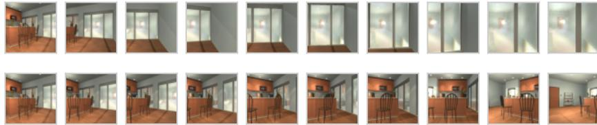
Figure 25: Orbit task. Top: The naive strategy looks directly at the reflective surface, causing tracking failure. Bottom: Filter-aware MPC avoids looking at the reflective surface.
