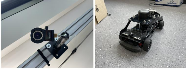
Figure 19: (Left) Optitrack camera. (Right) QCar. Markers placed on the QCar allow tracking the car's location and orientation through the OptiTrack system.
