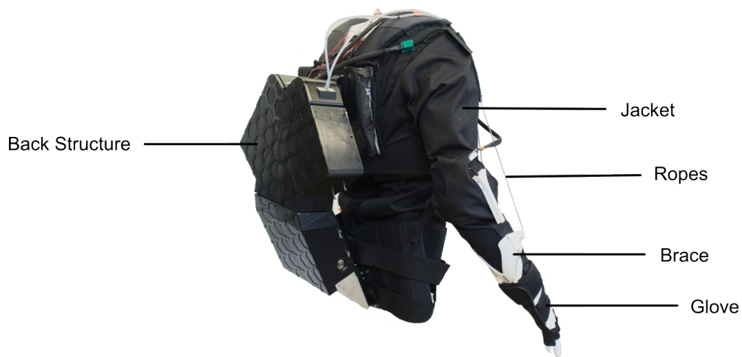
Figure 9 Final laboratory prototype of case study 1 without the FSR sensor strap. The black underlying jacket showcases the textile design (Section 7.3.1) and the rope design (Section 7.3.2) as result of the kinematic design of step 1, the back-structure and a brace at the forearm as part of the result of the pHMI Design (Section 7.4.2) in step 2 of the development process.
