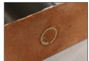
Fig. 3. Two different contact probes with their wafer-shaped tip geometry (a, b) and the laser-welded contact as a benchmark (c).
