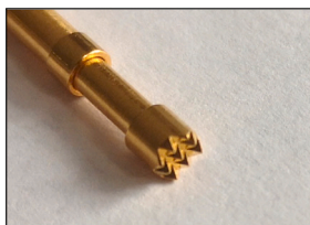
Fig. 3. Two different contact probes with their wafer-shaped tip geometry (a, b) and the laser-welded contact as a benchmark (c).
