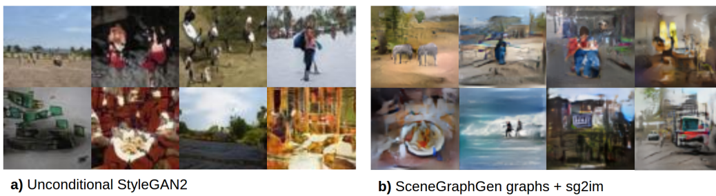
Fig. 10.5. Image synthesis examples with 64x64 resolution using a.) Unconditional StyleGAN2 trained on Visual Genome (left) b.) SG2Im on scene graphs generated by SceneGraphGen trained on Visual Genome (right).
