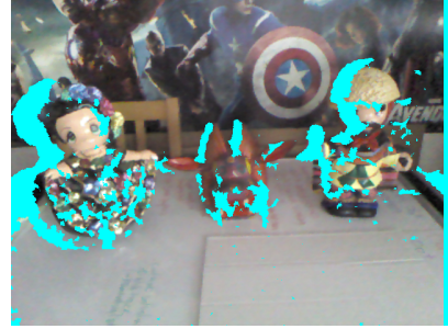
Figure 2.5: Kinect RGB-Depth overlapped image. Basically due to the difference in focal lengths ( f_{IR} > f_{RGB} ) the RGB and Depth image data do not fit: the cyan-colored areas of non-valid IR-depth values do not correspond to the object shapes of the RGB image.
