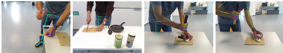
Figure 3.27: Examples of OP fragmented and failed detections under partial body visibility in some 2D scenes.
