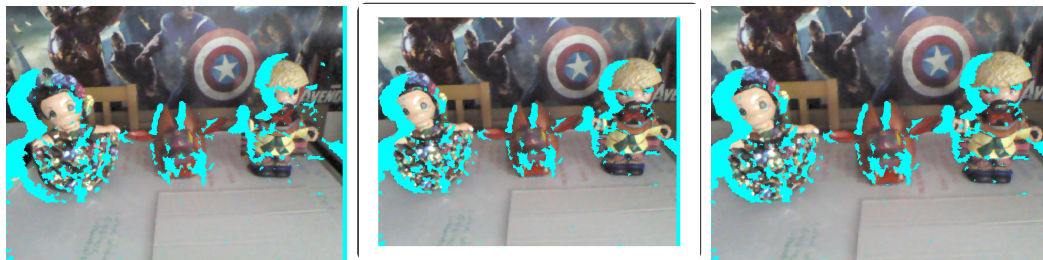
Figure 5.3: Kinect RGB-Depth overlapped and warped images. Basically due to the difference in focal lengths ( f_{IR} > f_{RGB} ) the RGB and Depth image data do not fit as can be observed on the RGB-Depth overlapped image (right), where the cyan-colored areas of non-valid IR-Depth values do not correspond to the object shapes of the RGB image. In the 1st adjustment, warped-Depth projected onto RGB (middle), we take the RGB as base and distort the Depth to fit the RGB image, observe that the resulting image is cropped to cover only the area overlapped by both images; In the 2nd correction, warped-RGB projected onto Depth (right), the base is the Depth image in which the warped texture of the RGB image is projected.
