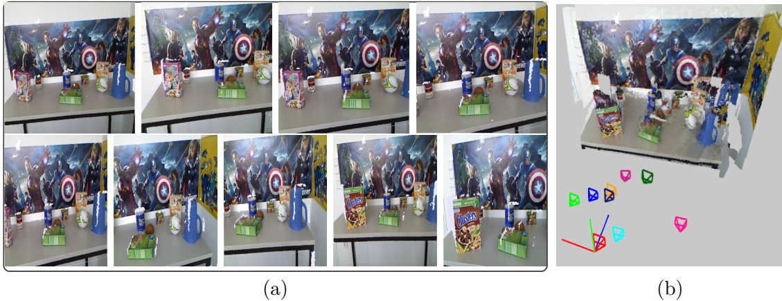
Figure 5.6: Exemplary mapping sequence for characterization of octree-DS performance. a) Individual 3D scenes, b) collated scene showing the camera poses from where each individual scene image in (a) was taken.
