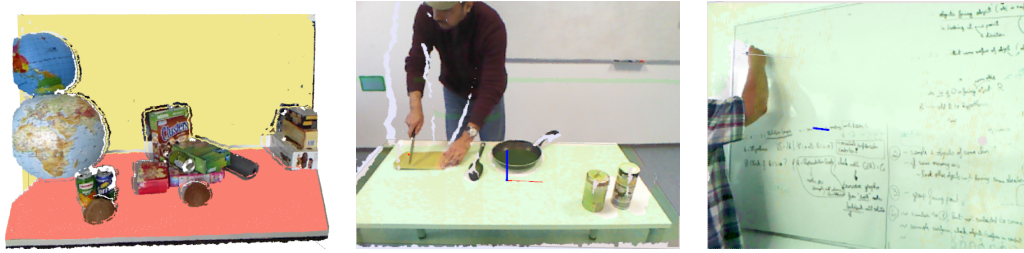
Figure 3.7: Geometrical detection of background regions. (left) Wall and table planes are found by repeatedly running ransac over the entire scene points (1st procedure); in the framework, supporting or interacting surfaces like a cooking table (middle) or a whiteboard (right) are determined by picking three plausible plane points on the image (2nd procedure).
