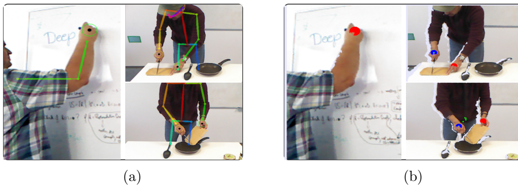
Figure 3.26: Augmented OP skeleton of hand-blob key points. a) Augmented hand-blob key points by extending the arms at the wrist sides in 2D images, the hand key points are marked with blue points inside yellow circles, b) the corresponding 3D spots of the 2D hand-blob key points are marked in the 3D images.
