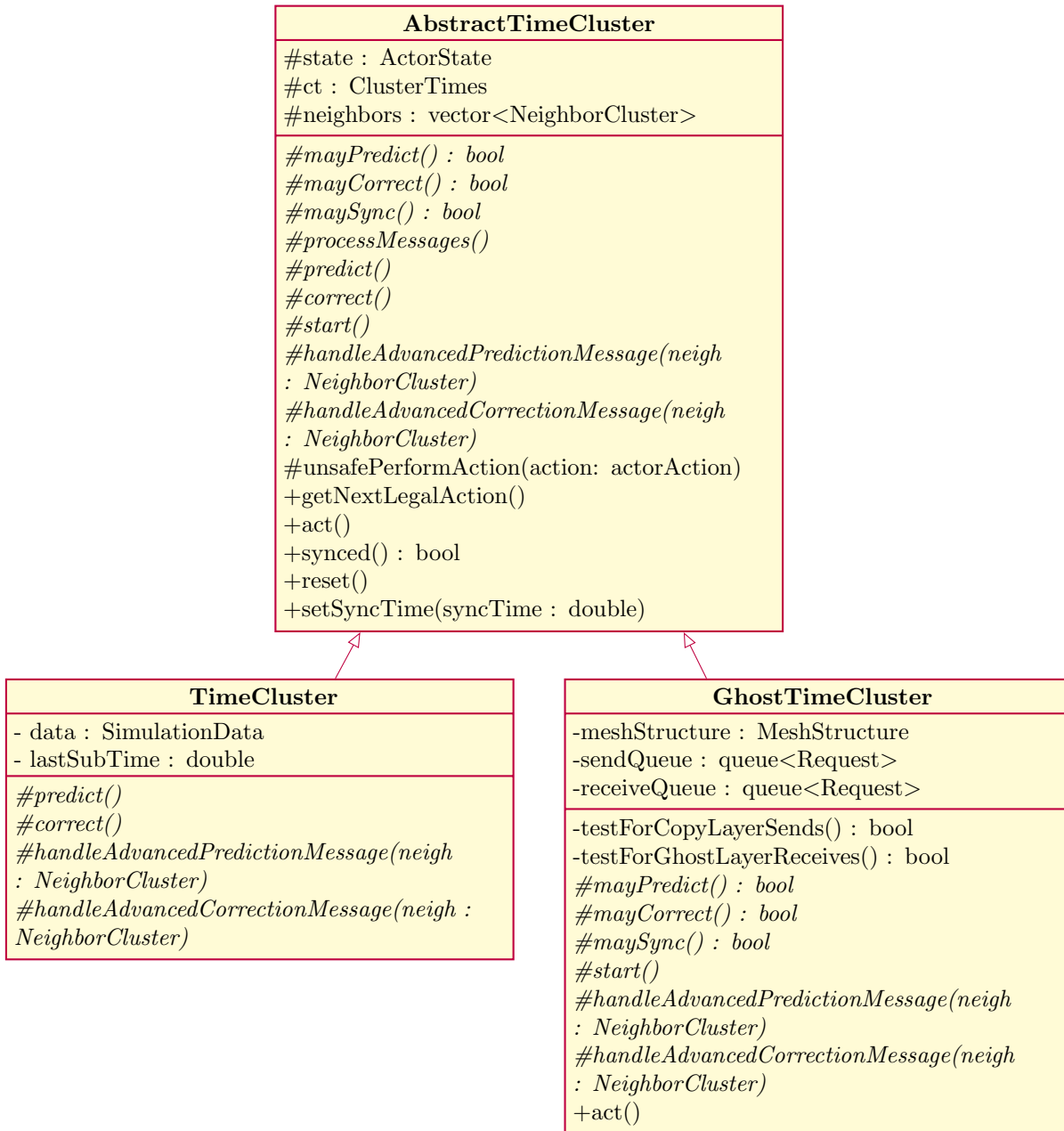
Figure 6.5.: UML class diagram that shows the structure of the TimeCluster and GhostTimeCluster classes, which inherit their functionality from the superclass AbstractTimeCluster . The attribute ct stores the local counters ( \Omega ), and the vector neighbors contains the shadow counters for neighboring clusters and the message queues. The variable data is a placeholder for the simulation data (e.g., the numerical solution and buffers required by LTS), and the variable meshStructure stores how neighboring ranks are connected. We assume the abstract superclass provides empty implementations for methods such as predict and correct . Note that both subclasses share the logic for act . Hence, they follow the same state machine. Note that the ghost time cluster tests for sends and receives in act to ensure MPI progression.
