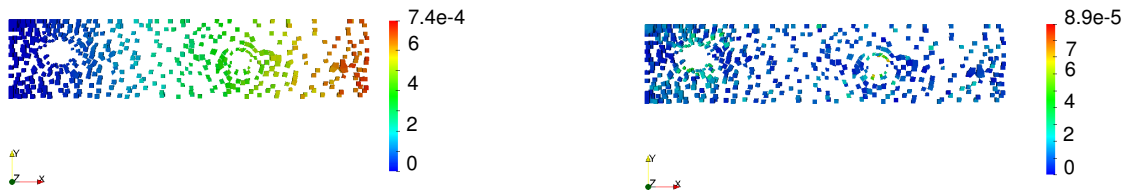
Figure 6.6 Resulting displacements in mm computed by the reduced order model (ROM) on the bottom and hyper-reduced (HROM) model on the top (for a fibre deviation field shown on the left of Fig. 6.5).
