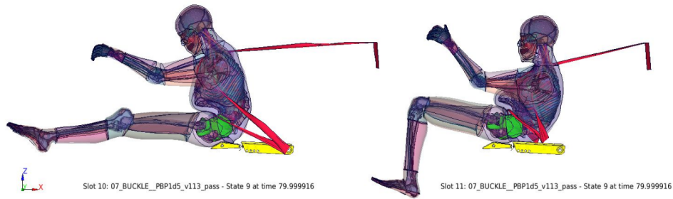
Figure 1.1 Human Body Model (THUMS, version 5, (Iwamoto et al, 2002)) in a frontal impact situation (Uriot et al, 2015) analysed with LS-Dyna to investigate submarining (Go, 2021).
