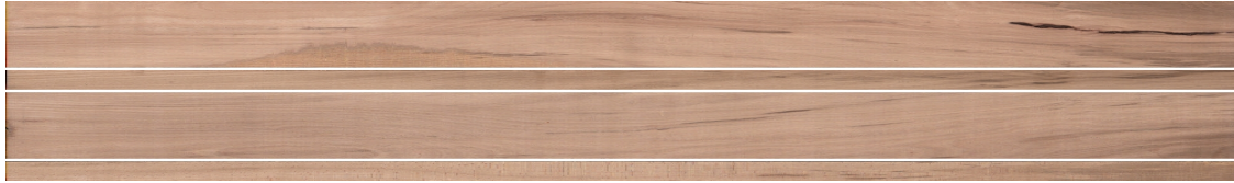
Figure 6.2 Exemplary beech board with varying fibre direction along the board, resulting in inhomogeneous material properties.
