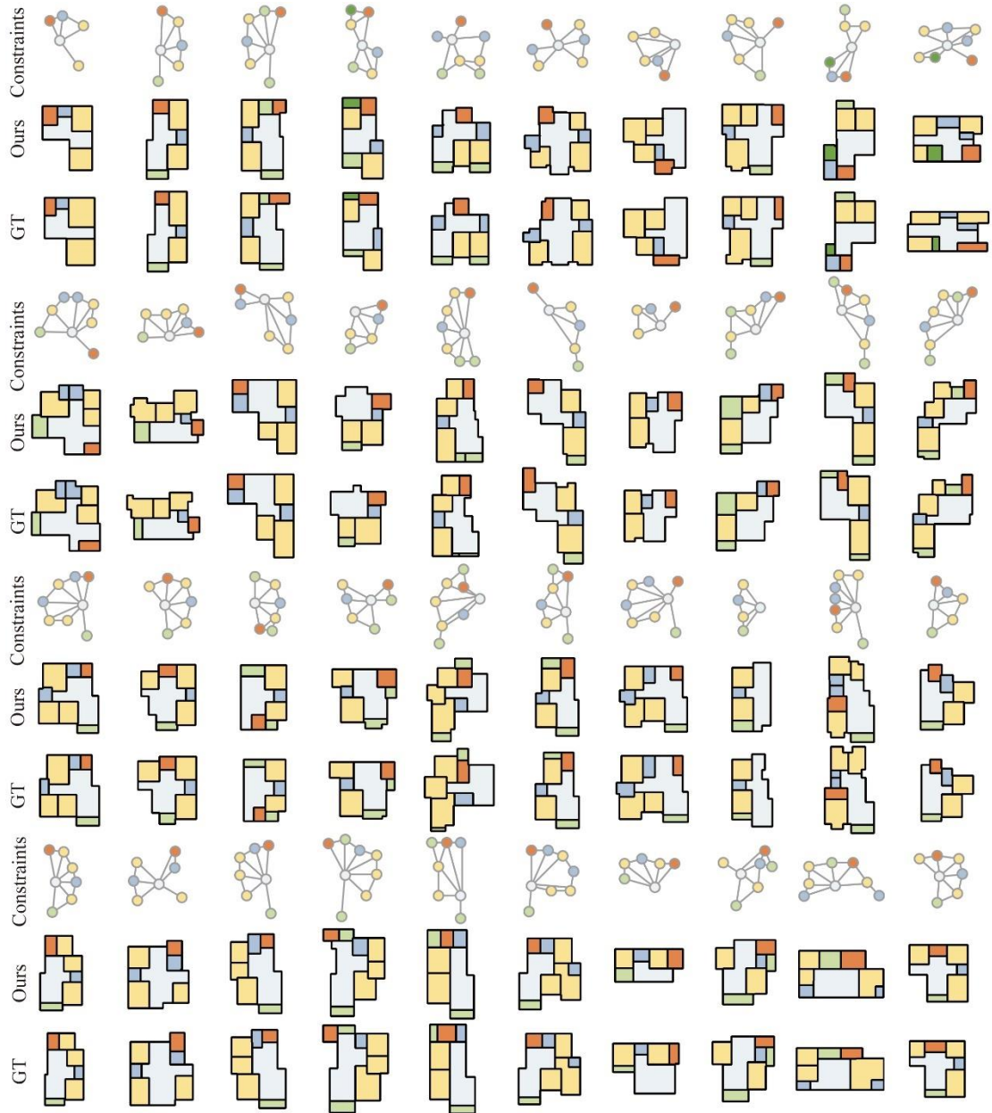
Figure 49 More generated room layout diagrams with the given bubble diagrams in the test split of RPLAN dataset.
