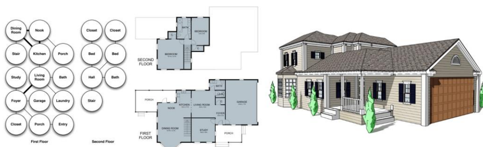
Figure 6 In traditional building design processes (Lu et al. 2017, Merrall et al. 2010)), especially in residual building design, the room functions and relative positions are determined with bubble diagram. All following steps are designed with the requirements in the bubble diagram.
