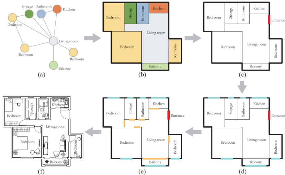
Figure 2 Hierarchical floorplan design process, in which the room layout design is the up-stream task. (a) Bubble diagram. (b) Room layout design. (c) Entrance design. (d) Window design. (e) Door design. (f) Fine drawn floorplan.
