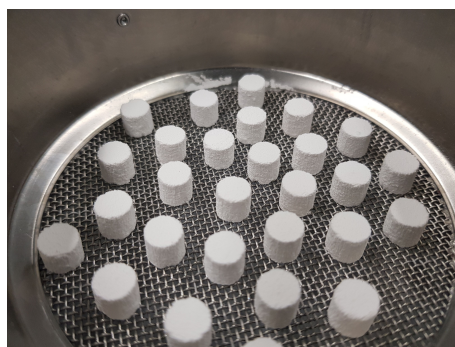
Figure 4.2: Debinded alumina cylinders placed on a stainless steel grid before post-processing.
